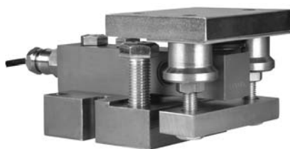
2-Directional 52-13 with base plate, lift off protection and upper welding plate
